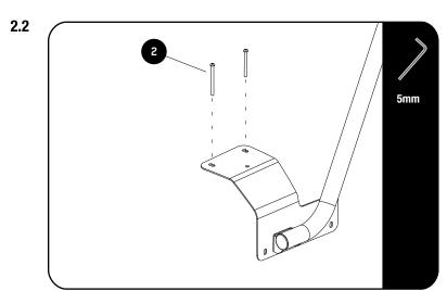
Apply a small bead of Thread Lock on the thread around the tip of the M6x80 Cap Screws (Item 2).
