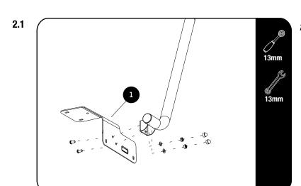
Assemble the LH Cowling Bracket (Item1) FAJL004 using two M8x16 Button Head Screws, two M8 Flat Washers and two M8 Nyloc Nuts (Fasteners also supplied with FAJL004).
