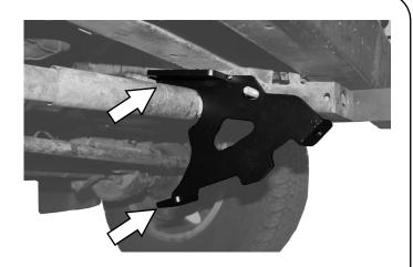
Place the Spacer over the Rear Hex Bolt and fasten loosely with it's respective washer and Nyloc Hex Nut.
