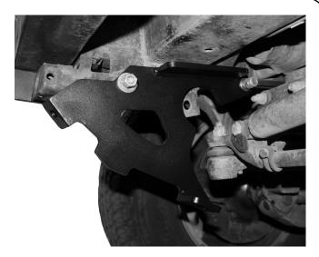
Now fasten the Sump Guard on to the Brackets with the Four M10 Counter Sunk Cap Screws, four M10 Flat Washers and four M10 Nyloc Hex Nuts (Items 3, 2 &1). Fasten the Sump Guard Fully.
