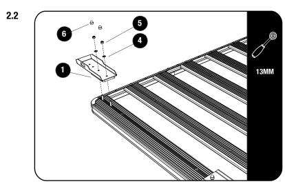
Fit the Gutter Mount Leg Extensions (item 1) loosley with two M8 flat washers (item 4) and two M8 nyloc nuts (item 5).
