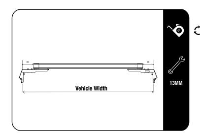
Adjust the Gutter Mount Extensions to suit the width of your vehicle.
