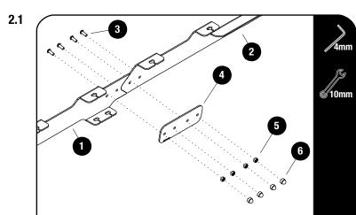
Assemble the front (Item 1) & rear (Item 2) foot rails using M6x16 button heads (Item 3), splice plates (Item 4) & M6 nyloc nuts (Item 5). Fully Tighten.
